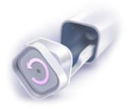
**Step 3.** We recommend waiting 1 minute before connecting the new case battery by twisting it back on.
